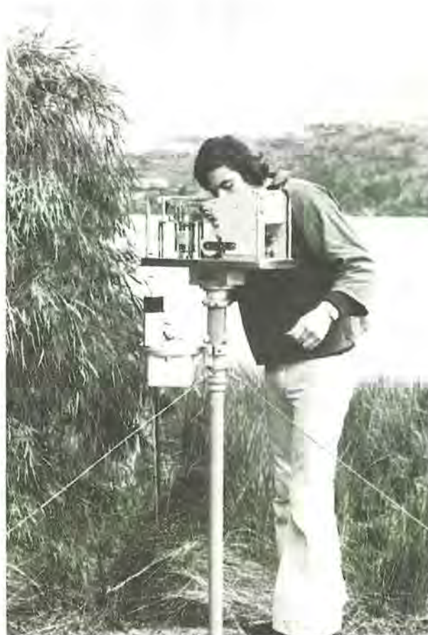
Recording tide gauge and barometer at Point Irwin. Mr. H. Agnew.
