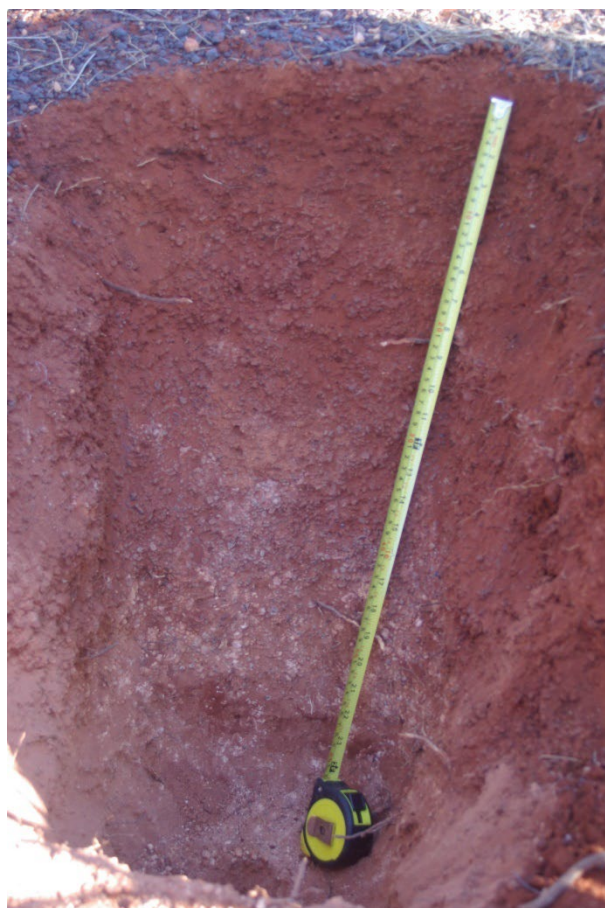
Figure 5.10: Calcareous loamy ironstone gravelly soil in the Moriarty land system – the subsoil (from about 30 cm to the base of the pit) has pale calcareous precipitation that ‘overprints’ the iron concretions; this was a common soil beneath Casuarina pauper (black oak)
