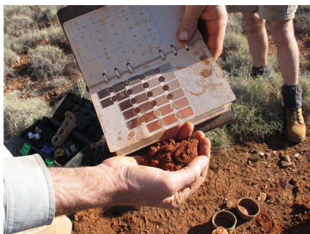
Determining soil colour by comparing a soil aggregate against a Munsell soil colour chart
