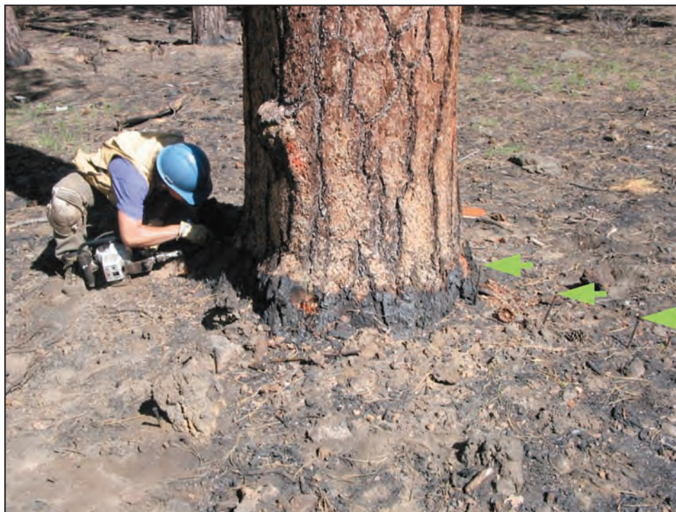
Figure 6. Using a drill to sample the base of a ponderosa pine for cambium kill after a prescribed burn. The charred, blackened area around the tree indicates the amount of litter and duff consumption. Arrows indicate the top of the duff pins radiating out from the tree base that were level with the surface litter prior to burning.
