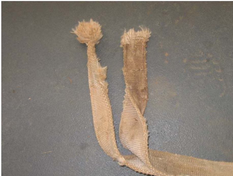
Damaged Snatch Strap
