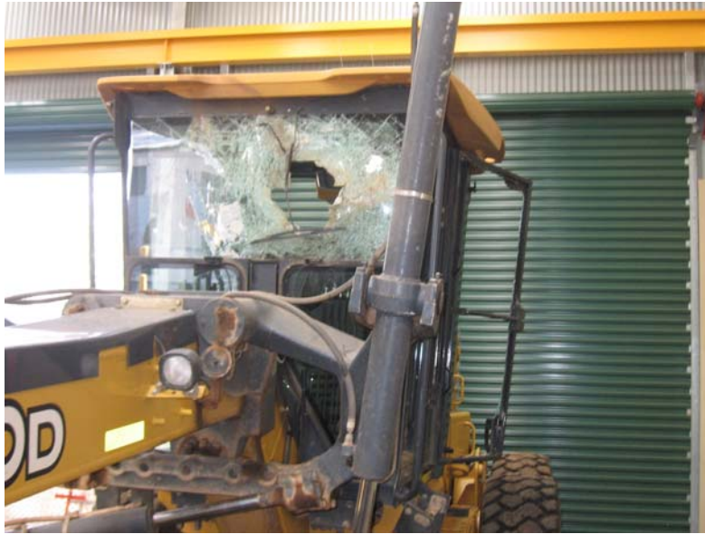
Damage caused by the snatch strap torn apart and ricocheting back into the graders windscreen. The operator of the grader suffered severe eye injuries from glass impact.
