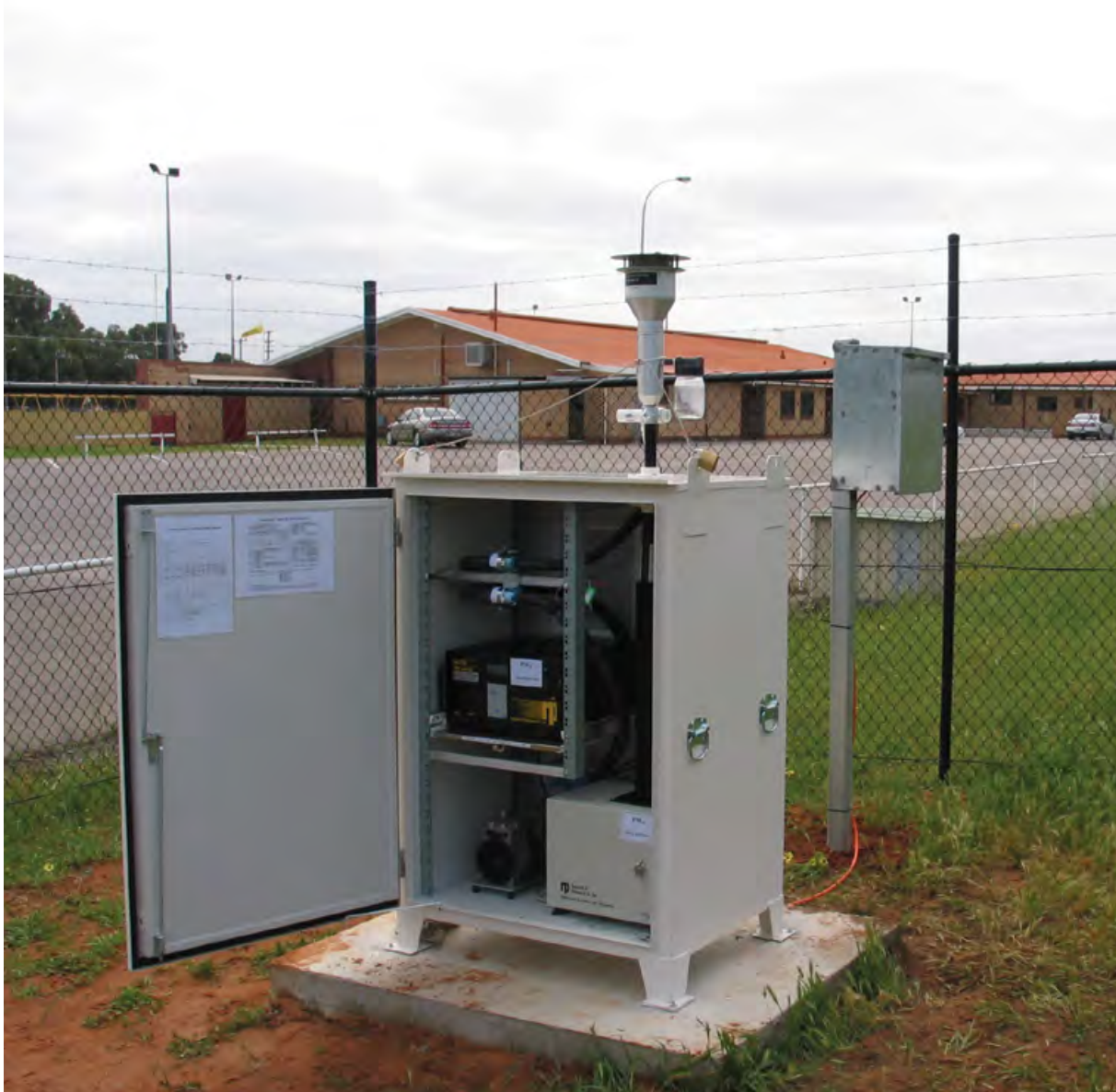
An ambient air quality monitoring station.
