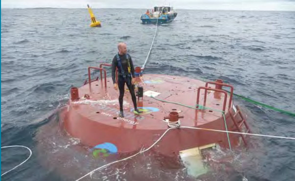
A buoyant actuator, part of Carnegie Wave Energy's wave power demonstration plant at Garden Island. Photo – Carnegie Wave Energy
