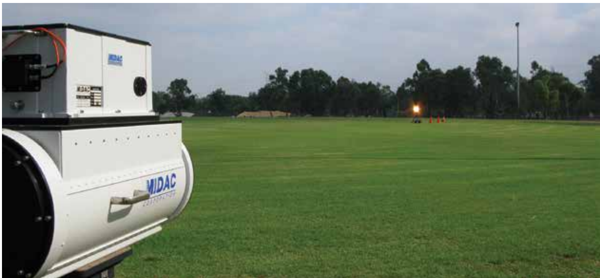
Fourier transform infrared monitoring equipment using a lightbeam, it can detect ammonia and organic compounds along an open path of between 60 and 100 metres.
