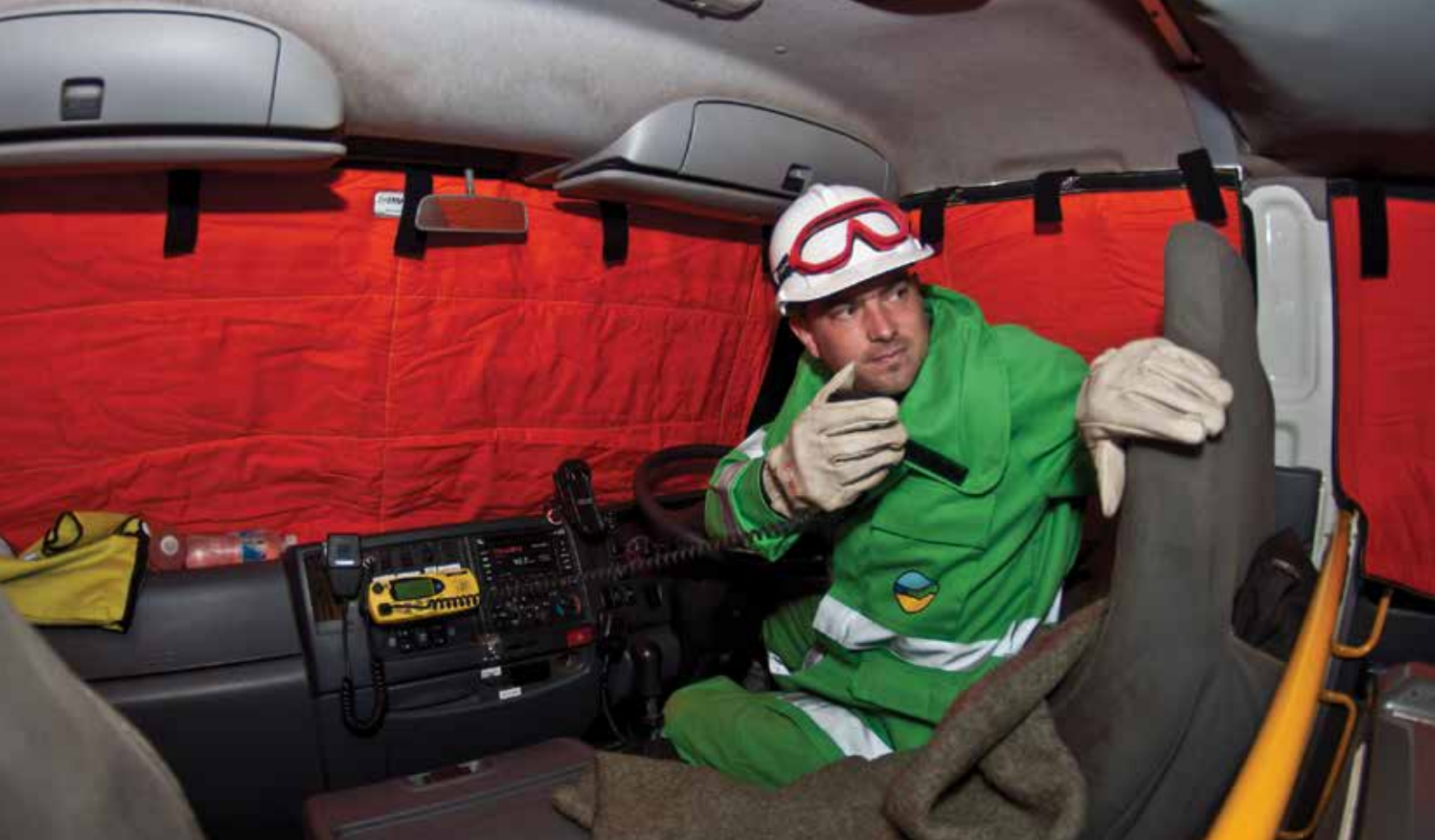
Tom Robinson checks the curtains installed in a fire truck. The curtains cover the windows to help protect crew from radiant heat in the event of them being caught in a burn-over. Photo – Peter Nicholas/DEC.
