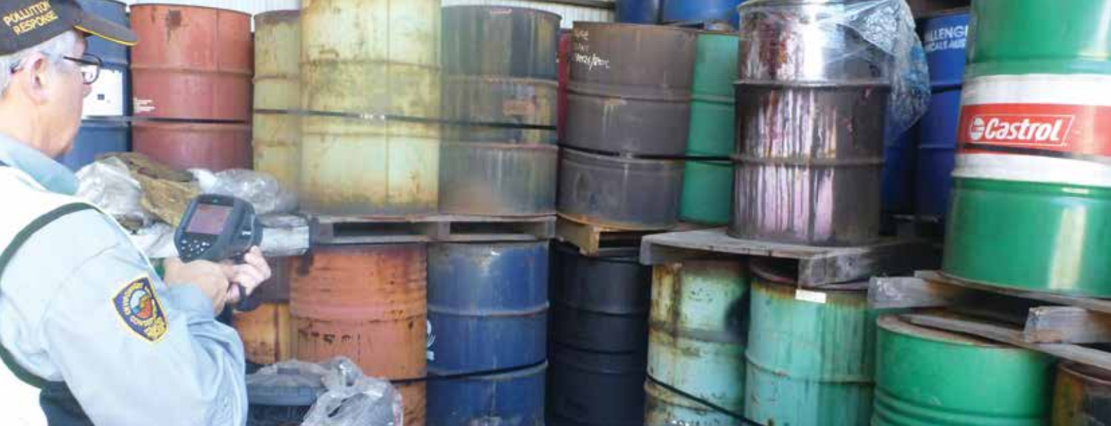
A DEC environmental officer uses a thermal imaging camera to assess chemical drums. Photo – DEC.
