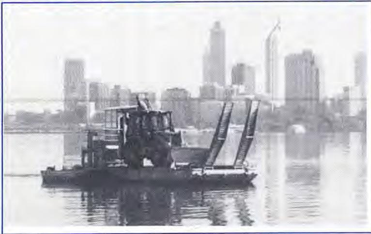
The barge 'Seagull', originally used to transport algae and weed between harvesters and shore unloading areas, has now been successfully converted to carry the Trust's heavy earthmoving equipment.
