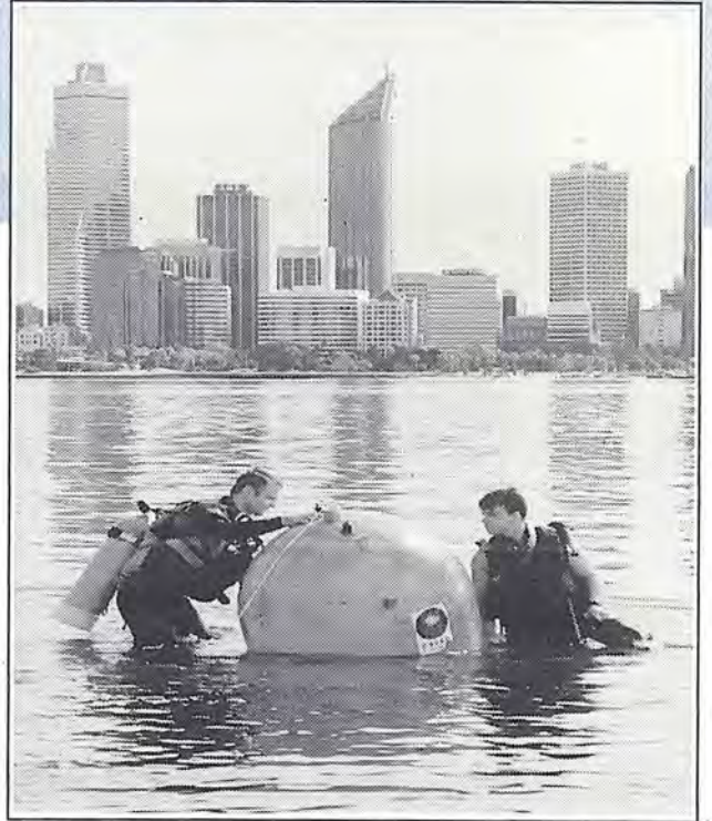
ABOVE To measure nutrient activity in the sediment of the Swan River, CSIRO used a large fibreglass dome to isolate sections of river bottom over periods of 4-5 days to replicate the process of deoxygenation leading to an algae bloom.
