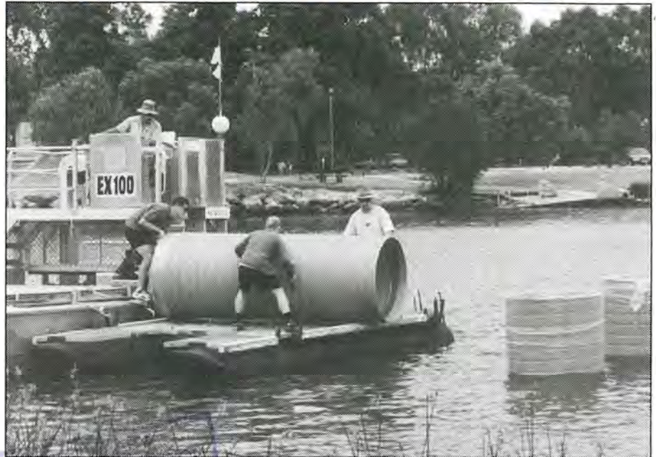
Swan River Trust field crew helped CSIRO staff place the 3m x 1m pipes into the river near Ron Courtney Island. Modified clay was added to the sediment at the base of each column to test the material's ability to remove phosphorus from the water column. During the two week sediment trial researchers conducted daily monitoring of nutrients, metals, oxygen, salinity and temperature.
