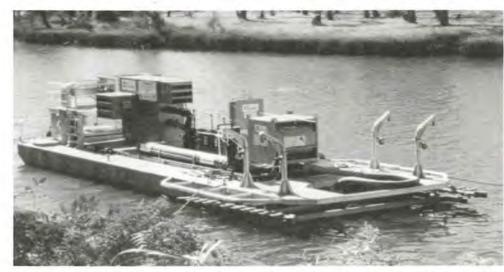
Around 200 kg of dissolved oxygen will be pumped into sections of the Swan River's middle reaches every day this summer as part of an innovative experiment to test the use of oxygen as a means of improving water quality in this environment.
