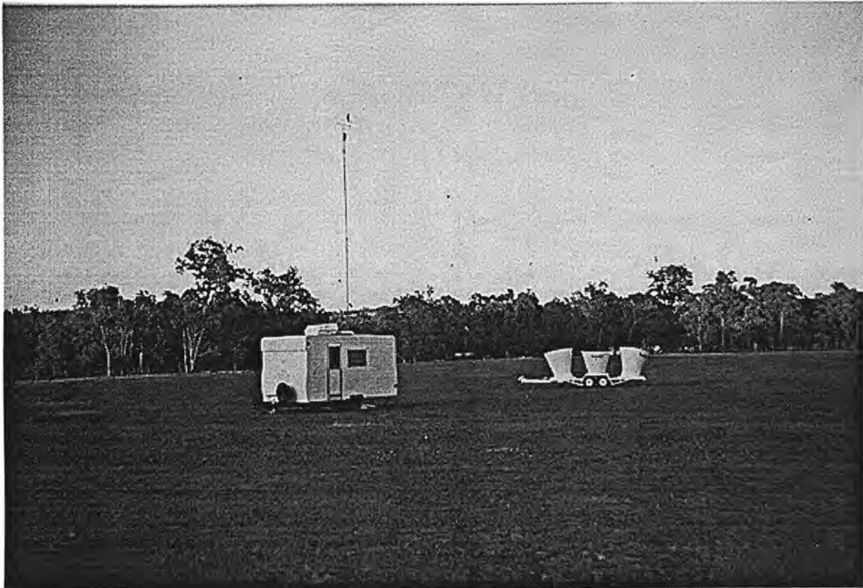
Figure 7.3 - Sodar equipment located at Gidgegannup.
