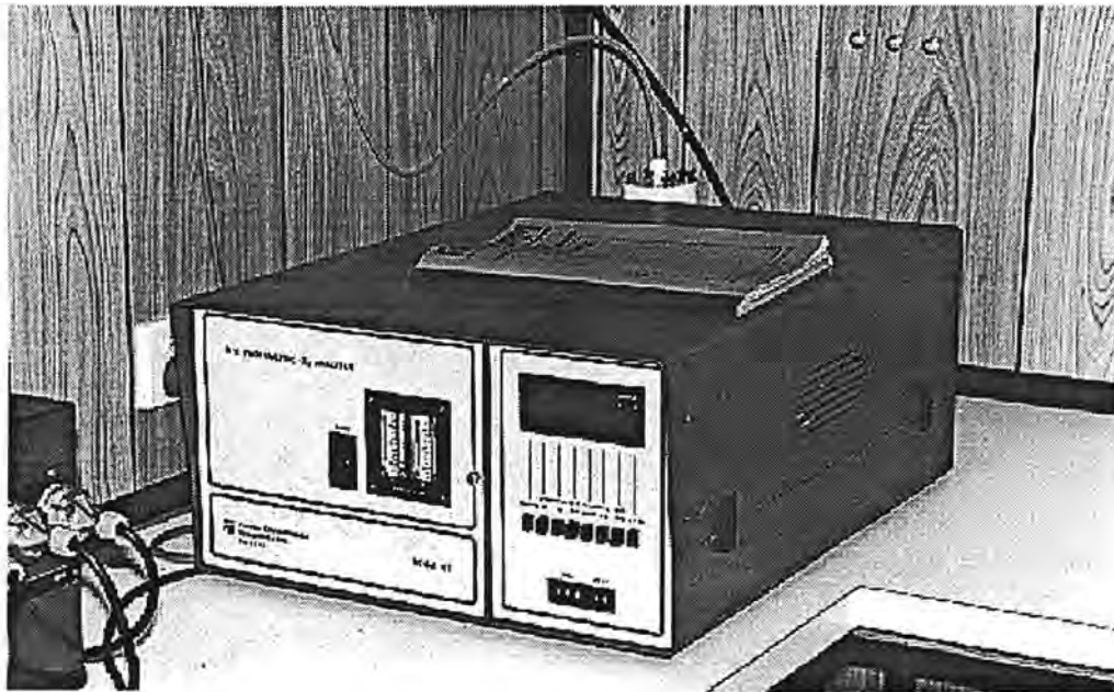
Figure 5.2 - Shed interior showing an ozone monitor with the site log book.
