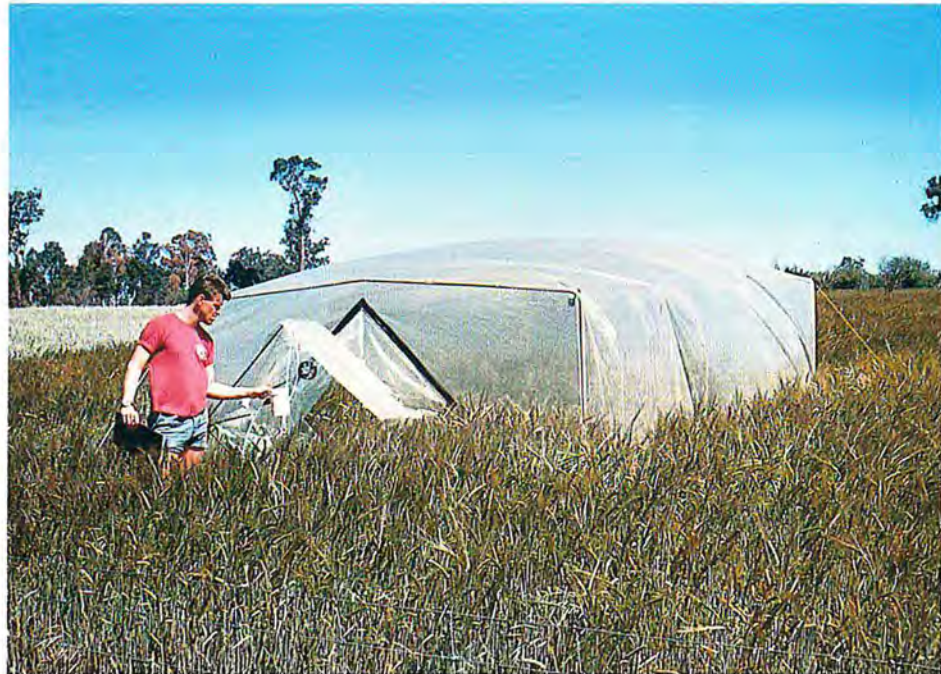
Ventilated chamber measures barley transpiration at Bowelling. Barley is one of a number of crops which has higher water use than traditional pasture.
