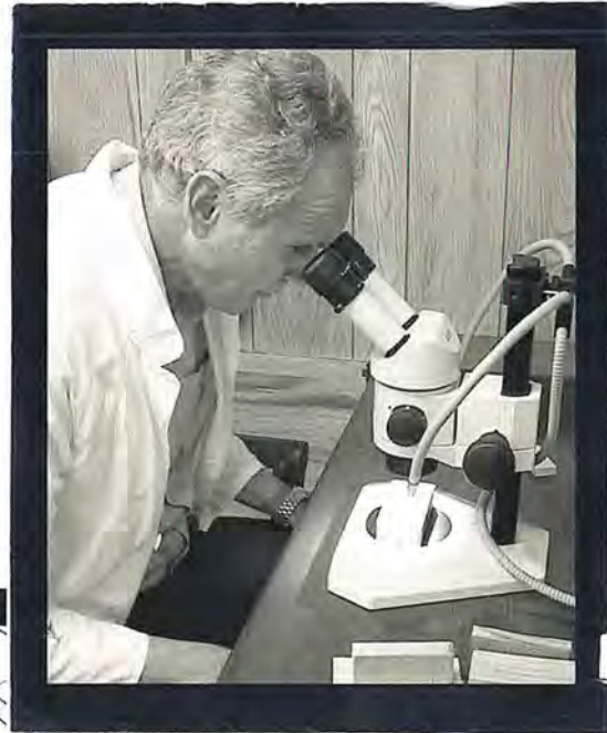
Dr Graeme Siemon, FPC Timber Scientist, studying the cell structure of radiata pine.
