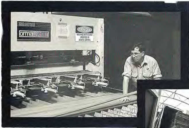
FPC Technical Officer Peter Piper is pictured edge gluing timber panels at the Timber Technology Centre.
