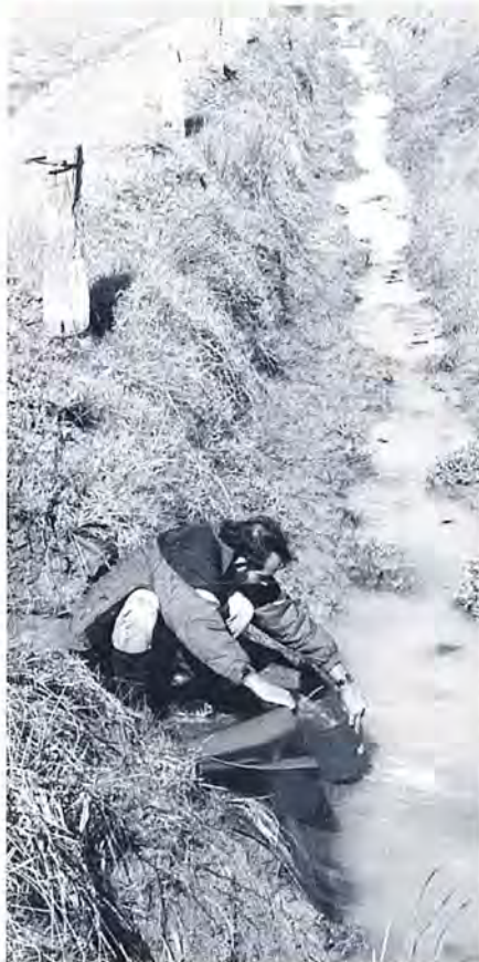
Big reductions in salinity and waterlogging ... Agriculture Western Australia hydrologist Don Bennett samples runoff at the sub-surface drainage trial at Bengier.
