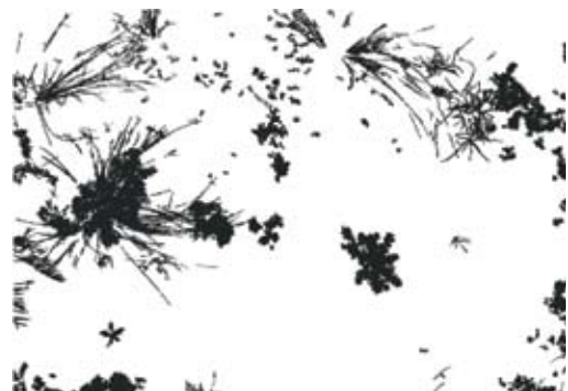
New method CMOS image. Litter, wood and shadows are erased making it easier to estimate coverage. Green foliage is black and background is white.
