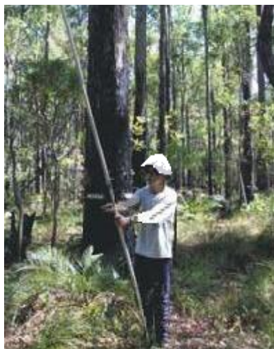
Gary Ogden taking a nadir image of understorey, using a bubble level pole. Camera is operated with an infrared remote control.
