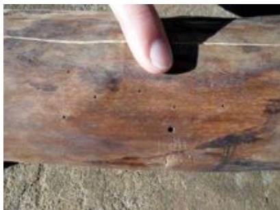
Different sized exit holes caused by borers. A weevil was extracted from the larger hole.
