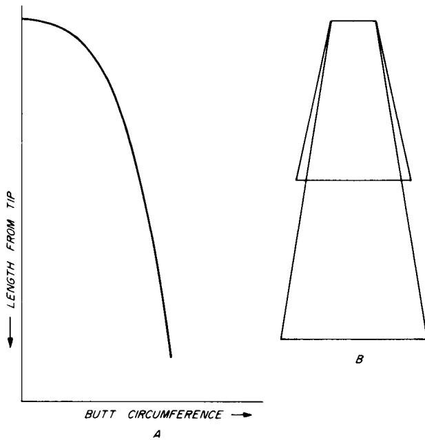
Figure 4.—A. The general relationship between length and butt circumferences of round timbers that are classed by the ANSI 05.1 standard. B. Profile of two poles of different lengths and with minimum tip and butt circumferences.
