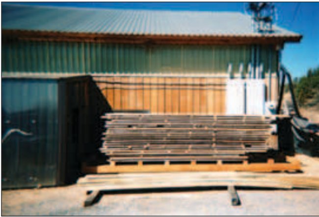
Figure 6—Stickered ponderosa pine lumber stacked on rail cart. Note poor lumber piling, spacing of stickers, and alignment.
