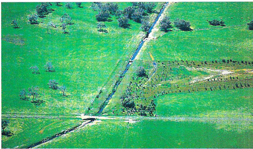
Water entering the Mealup Drain from this farm drain is made to pass through a vegetated area, which slows the flow and acts as a filter
