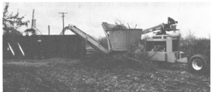
Figure 5--To increase biomass density, the material may first pass through a tub grinder, then into the module builder.
