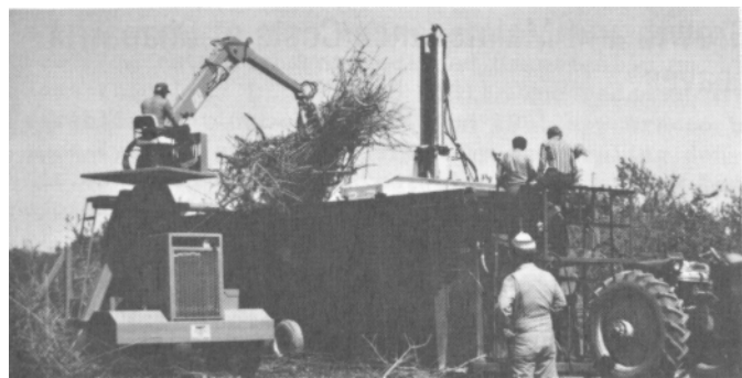
Figure 3--The biomass is placed into a module builder, adapted from the cotton industry, distributed and compressed into a unit 7½ feet wide, 30 feet long and 8 feet high.
