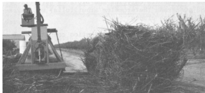
Figure 4--A free standing module, having a density of 8 to 10 lb /ft 3 , ready to be picked up by a transport vehicle.
