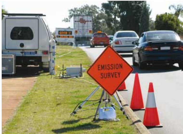
CleanRun RS measuring vehicle emissions in Balcatta
