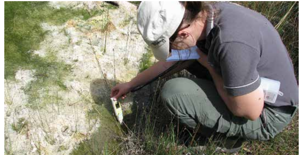
A Parks and Wildlife officer measures the pH and temperature of the water in a wetland near Cervantes. Photo – Parks and Wildlife
