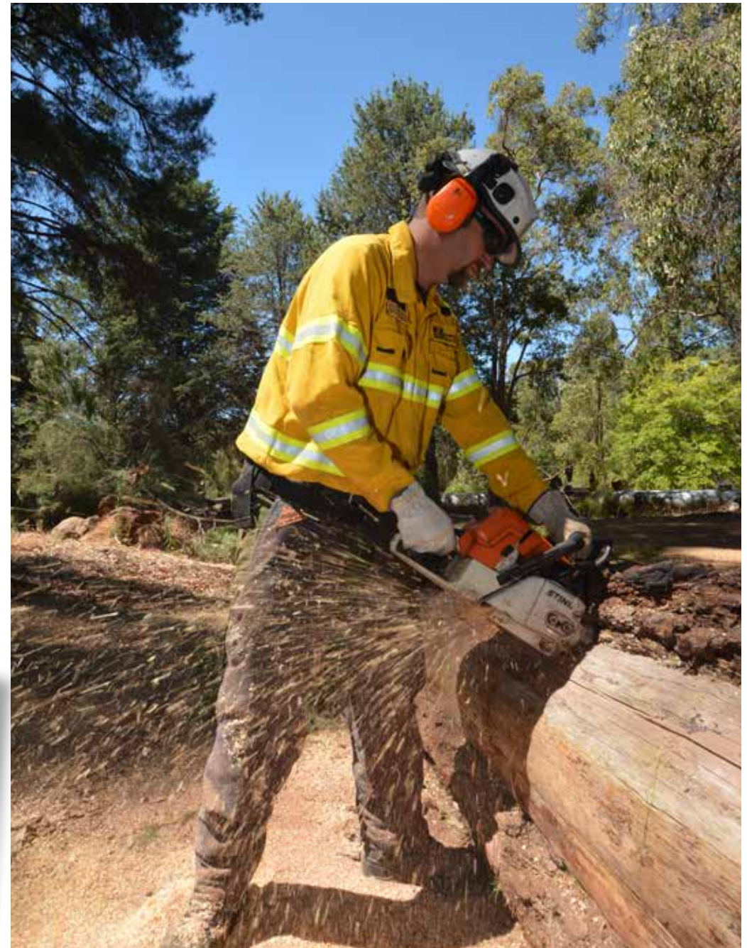
Conservation employee Paul Dunstan demonstrates the method and protective gear required to chainsaw safely. Photo – Peter Nicholas/Parks and Wildlife
