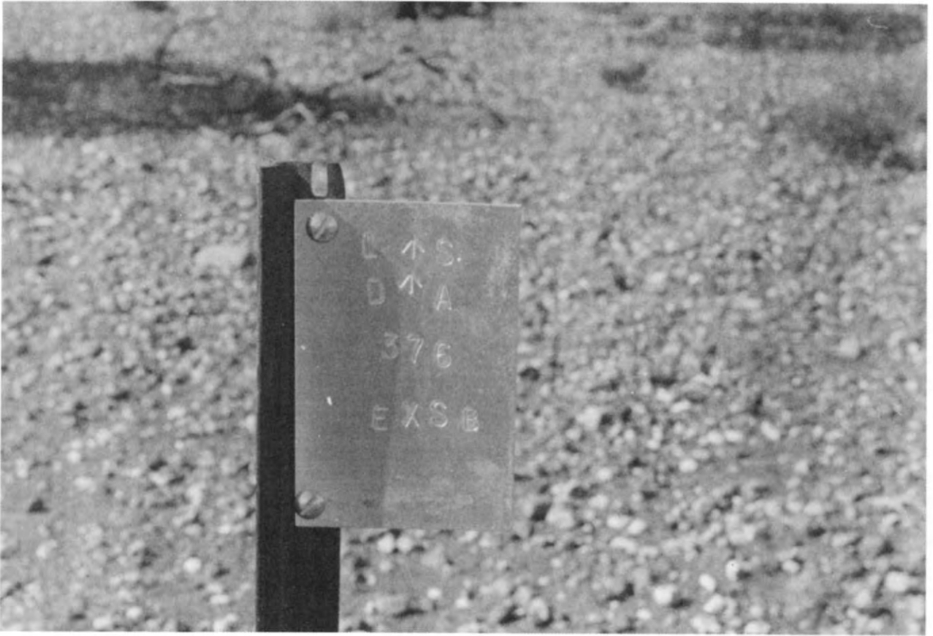
12. Each site was marked with an aluminium plaque which identifies the agencies, site number and survey code.
