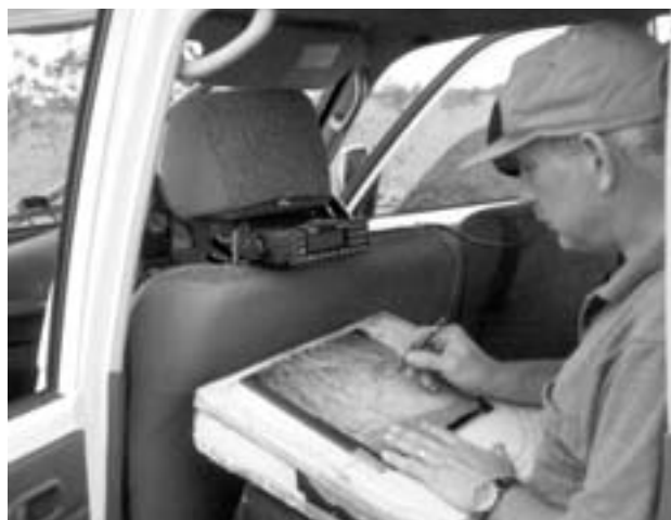
Verification of land system boundaries and station infrastructure with a GPS unit and aerial photography during traversing.
