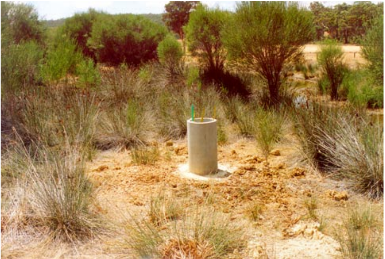
Photo 7: WW3 – Groundwater monitoring bore at the upstream property boundary.
