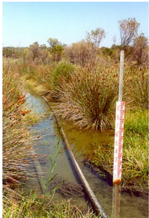
Photo 5: WW2 – Staff gauge for monitoring surface water levels in the wetland.
