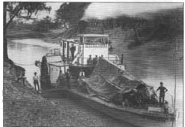
Plate 4. The paddle steamer Excelsior on the Darling River circa 1895, loading timber for fuel to fire the boiler.
