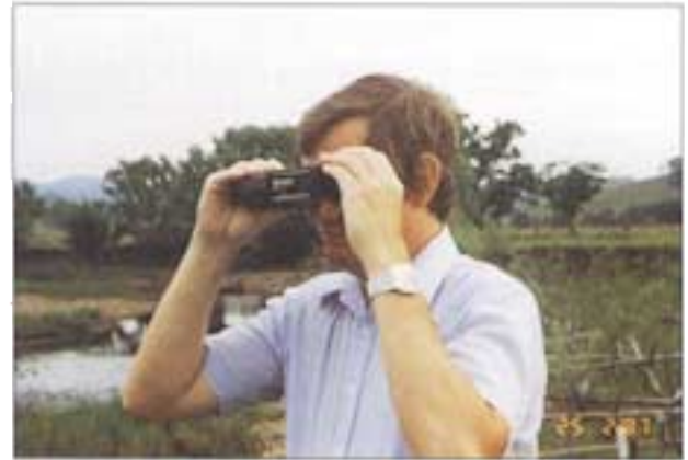
Plate 10. By using an optical range finder, channel widths can be quickly compared with the ideal and an assessment made of the degree of degradation.
