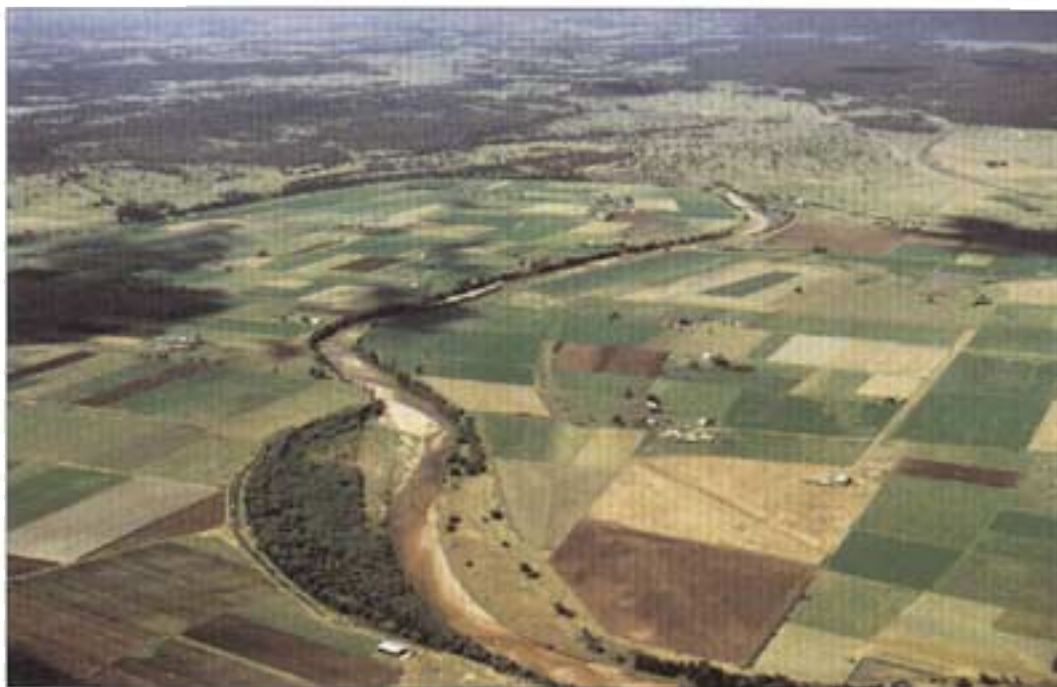
Plate 9. Photograph taken from the left bank of the Hunter River at Scotts Flat, looking downstream. It shows the river being trained past an extensive eroding bank from stable section to stable section. The river works are now well consolidated.
