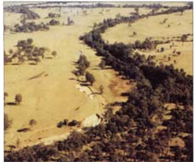
Plate 11. The Williams River looking upstream from below Dungog showing how a choked channel has forced water onto the floodplain, scouring a new channel. Judicious clearing of the main river, particularly the inside points, has remedied this potential diversion.
