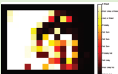
2d. Image processing algorithms showing the results of the classification of the sprayed Salvinia image. The legend on the right indicating the probability of a detected weed.
