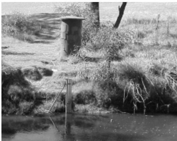
A low cost gauging station at Southern River, Anaconda Drive (accuracy of flow +/- 15%).
