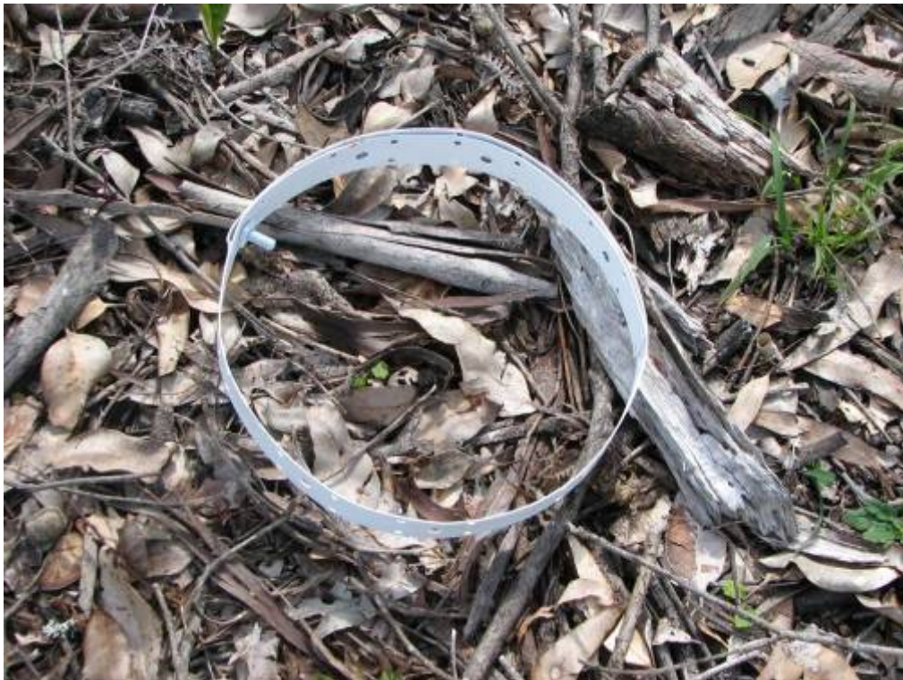
Undisturbed (D0) level of soil disturbance - characterised by an intact litter layer
