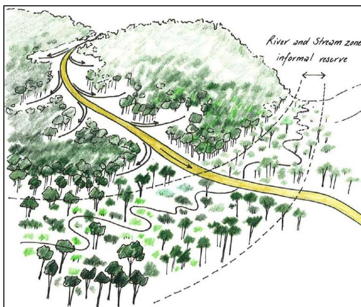
Figure 16: Mitre drains remove surface water at regular intervals to stable areas before the road enters an informal reserve. Install additional structures to control surface water in the informal reserve as required (within the road corridor).
