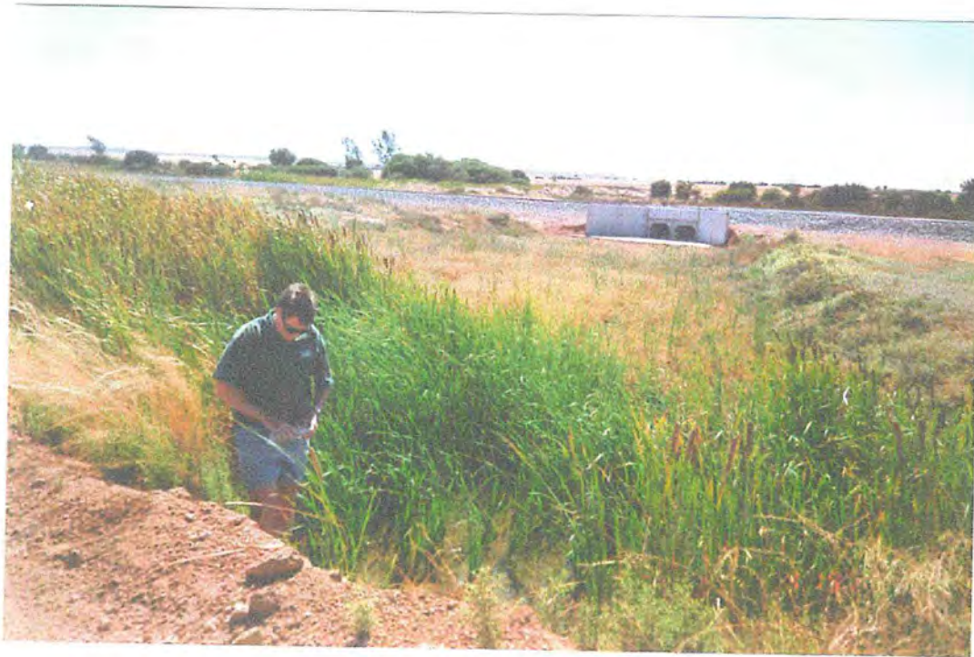
Photo 26 Eagle Hill Trib, viewed upstream/east. A tributary of the Coonderoo River. The presence of bull rushes indicates groundwater fed, all year round flow, 14/02/01. Salinity was 2,600mg/l in February 2001.
