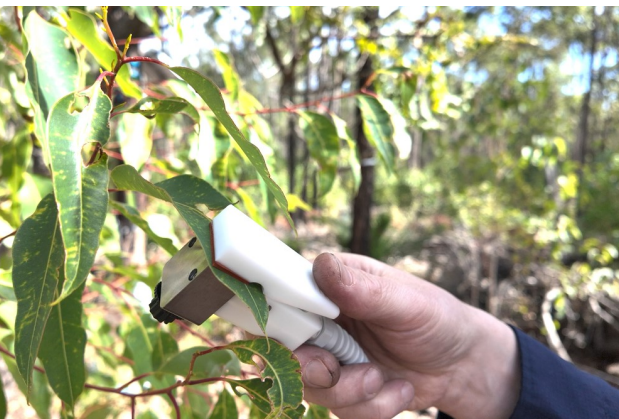
Top left: a slingshot is used extract leaves from high in the tree canopy to examine tree stress levels. Top right: measuring diameter helps map tree population structure, and understand how trees are growing. Bottom left: leaf porometer measurements are taken to check stomatal conductance (how well the tiny openings called stomatal pores on a leaf's surface are working to let gases in and out), which is critical for the plant's ability to make food and stay hydrated. bottom right: a short pronged soil moisture meter checks surface soil moisture which can inform how soil moisture is influenced by canopy density.
