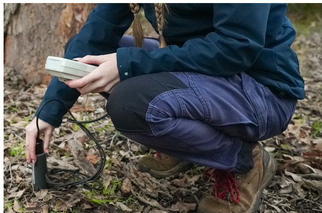
Top left: a slingshot is used extract leaves from high in the tree canopy to examine tree stress levels. Top right: measuring diameter helps map tree population structure, and understand how trees are growing. Bottom left: leaf porometer measurements are taken to check stomatal conductance (how well the tiny openings called stomatal pores on a leaf's surface are working to let gases in and out), which is critical for the plant's ability to make food and stay hydrated. bottom right: a short pronged soil moisture meter checks surface soil moisture which can inform how soil moisture is influenced by canopy density.
