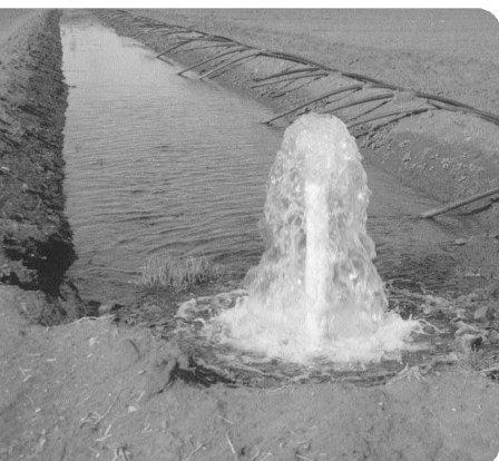
Test pumping discharge, Ord River Irrigation Area
