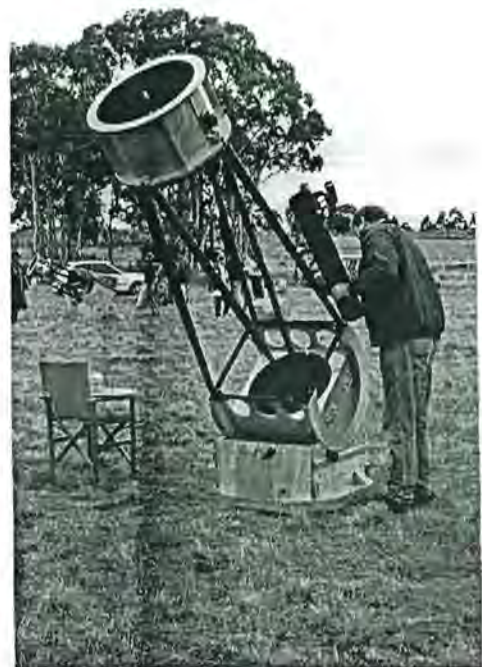
The largest telescope on the field was this 22" truss design Newtonian – all home made. Joss (the owner) is just putting on the finder.
