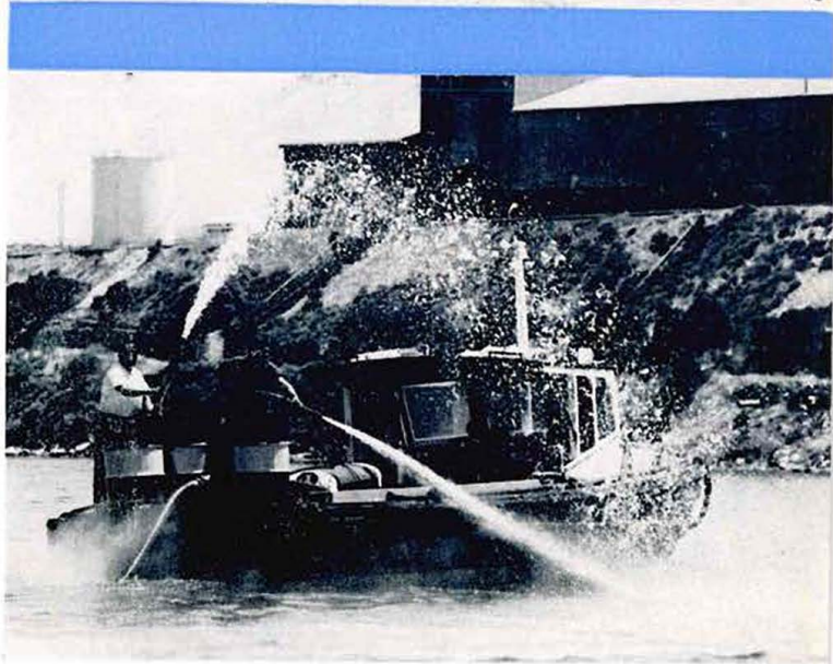
Fremantle Port Authority tender breaking up oil film at Preston Point, with detergent sprays.
